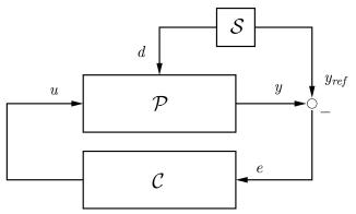
Consider a System  $\mathcal{P}$ , a Signal Generator  $\mathcal{S}$  and a Controller  $\mathcal{C}$  where y is the Output and e the Regulation Error.
