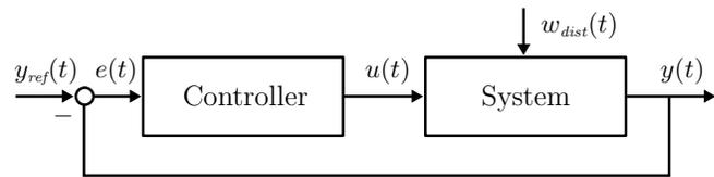
Fig. 1. Dynamic error feedback control scheme.
