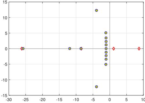
Fig. 2. Spectra of the uncontrolled system (red diamonds) and the closed-loop system with  $r = N = 300$  (yellow stars) and  $r = 12$  (blue circles).
