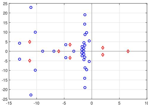
Fig. 6. Spectra of the uncontrolled system (red diamonds) and the closed-loop system with  $N = 1258$  and  $r = 12$  (blue circles).
