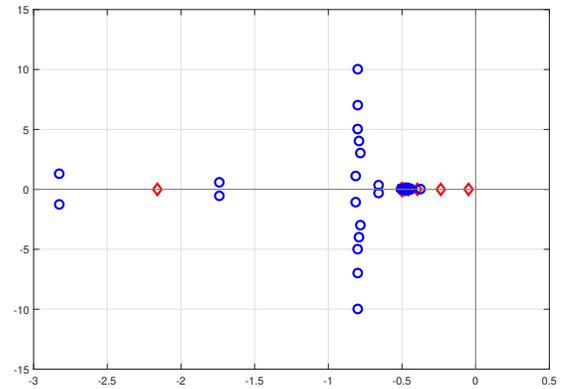
Fig. 8. Spectra of the uncontrolled system (red diamonds) and the closed-loop system with  $N = 58$  and  $r = 10$  (blue circles).
